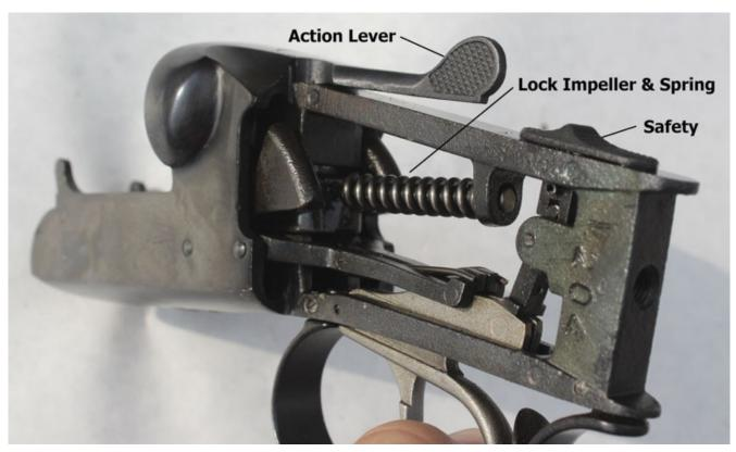
2. **Shortening the lock impeller spring** The spring around the lock impeller is stiff and requires a lot of pressure on the lever to break it open. Removing some of the spring makes it easier (and faster, the real reason) to open the shotgun. At the same time I was shortening the rod, I was also
